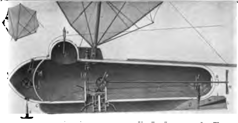
Sectional View of the Nautilus
